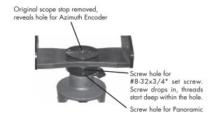
Azimuth encoder in position. Note how Main Wiring Harness is draped through the Yoke and Cradle
